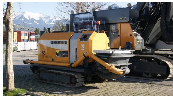
Figure 12.11 – Fixed Pumps generally have the Highest Pumping Capacity and are the usual Choice for Major Projects 12.5
