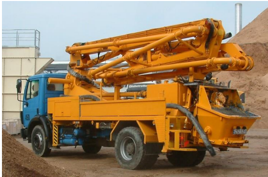
Figure 12.12 – Mobile Concrete Pumps are quick to Set up and Versatile in their Range of Applications 12.6
